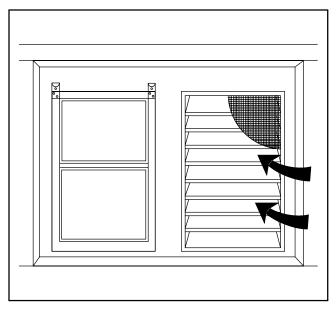
Figure 4-3 Stationary Louvers for Air Inlet
